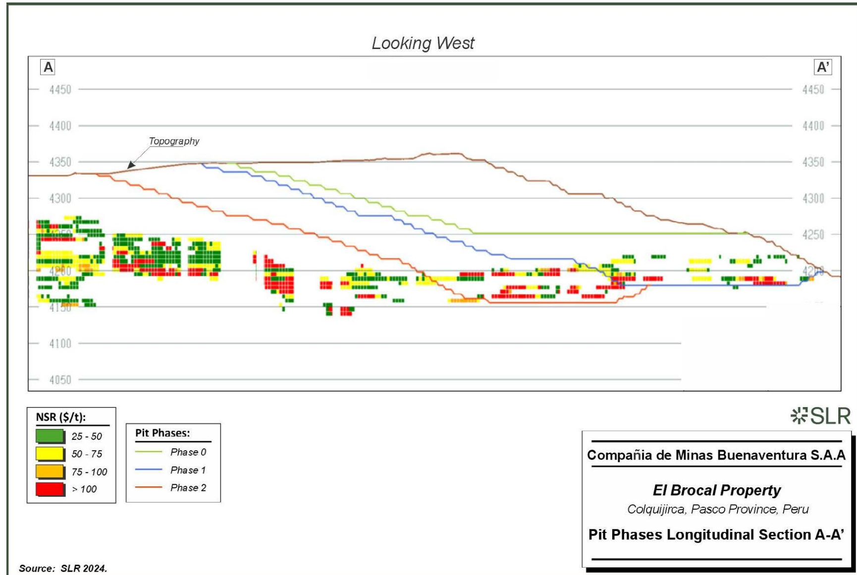
Figure 13-9: Pit Phases Longitudinal Section A – A'
