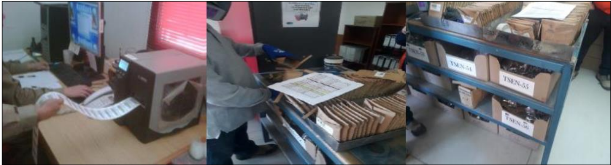
Figure 8-10: QA/QC Samples Insertion; A) Label Printing from acQuire; B) Labelling of Pulp and Checking of Position of Controls According to scheme of analysis; C) Control Types
