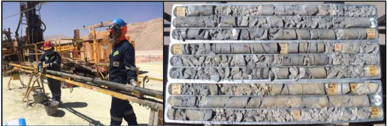
Figure 8-2: DDH Sampling; A) Sample Collection; B) Sample Distribution in Metallic Trays
