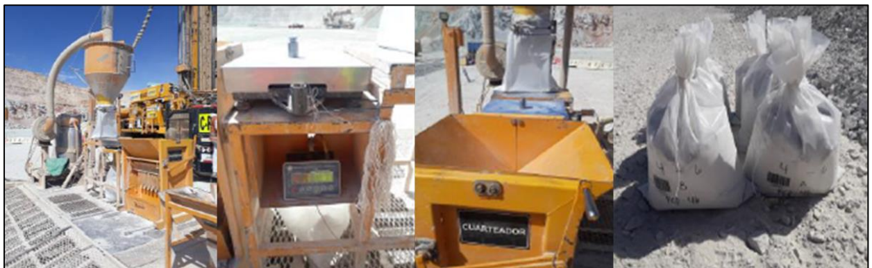
Figure 8-1: RC Sampling; A) Sample Collection; B) Weight control; C) Sample Splitting; D) A and B Samples
