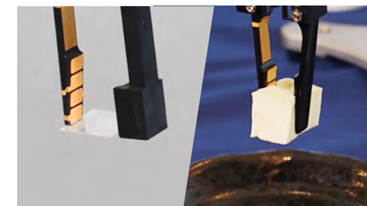
MoR® picking up a microscope slide and a piece of soft tofu
