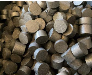
Metal chips or shavings are compressed to make them easy to reuse
