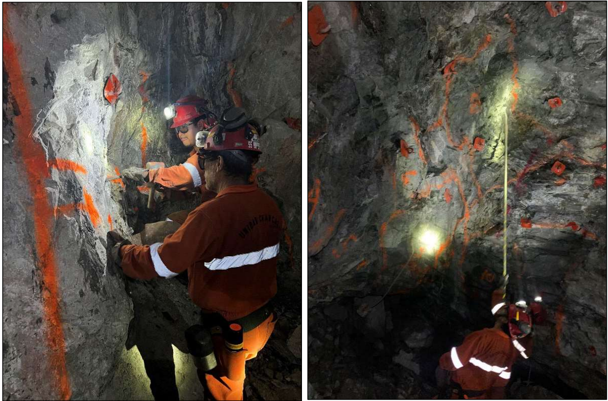
Figure 7-4: Rock Sampling using Hammer and Chisel (Left) and Long Bars (Right)
