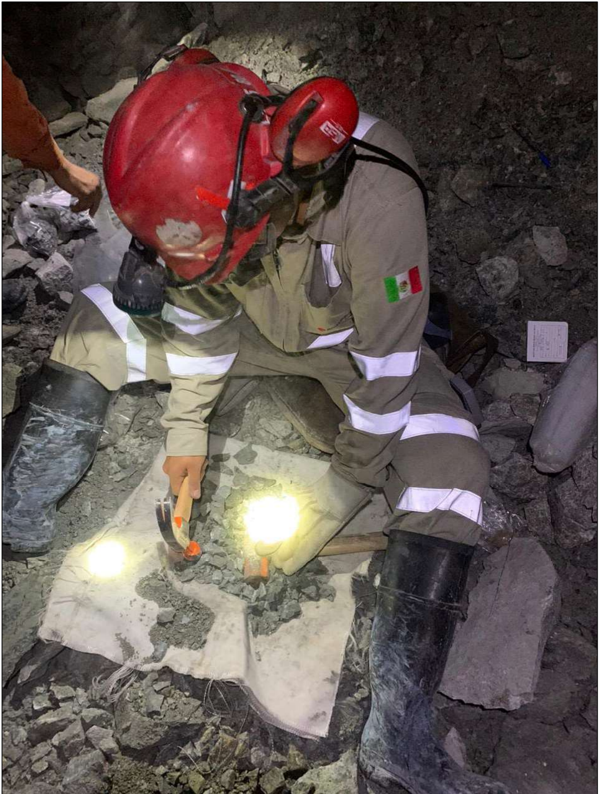
Figure 7-5: Homogenization Process of Sample Particle Size
