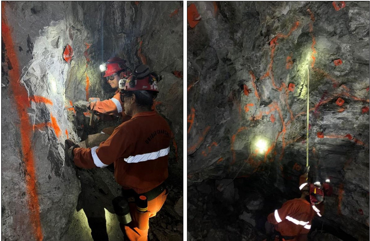
Figure 7-3: Rock Sampling using Hammer and Chisel (Left) and Long Bars (Right)
