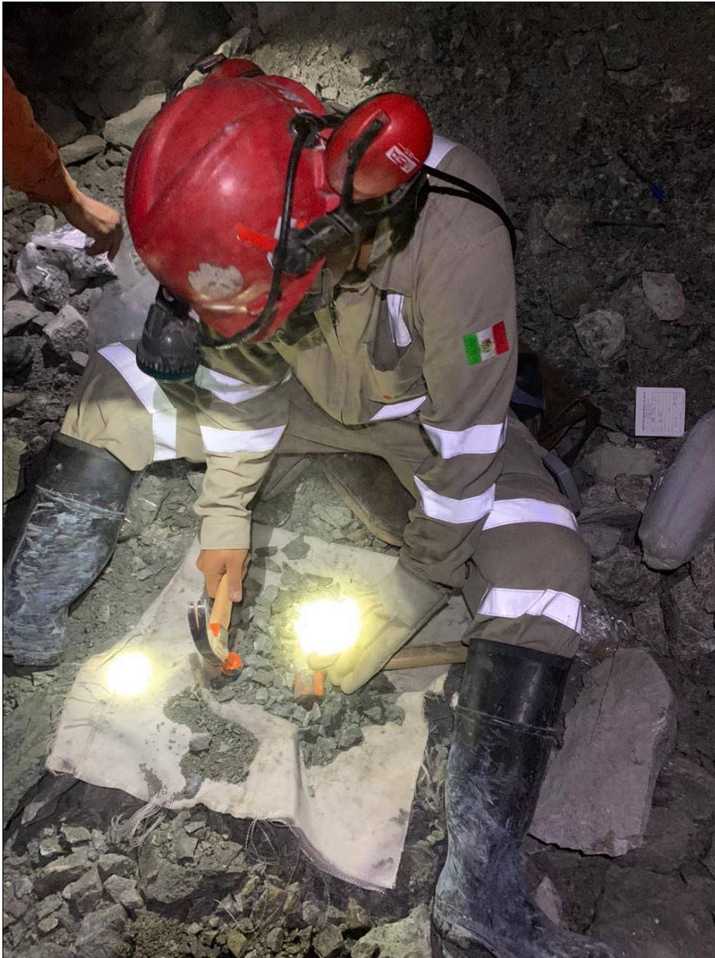
Figure 7-4: Homogenization Process of Sample Particle Size
