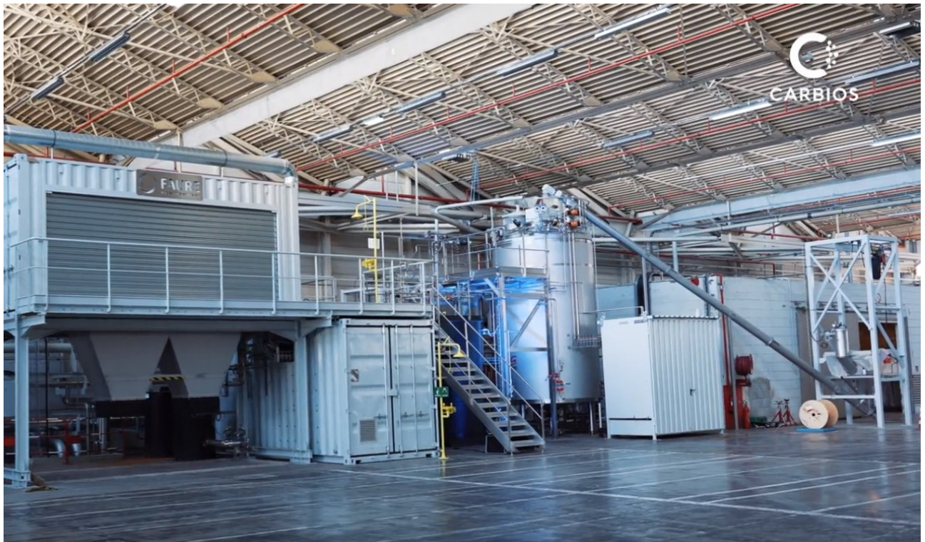
Pre-industrial unit dedicated to the depolymerization of PET plastic and textile waste into monomers. (Carbios)
