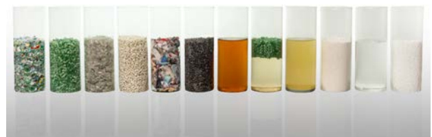
Depolymerization of PET plastic waste to form terephthalic acid (TA) and monoethylene glycol (MEG) in a hydrolysis reactor and the repolymerization of these monomers into food quality PET, 100% recycled and 100% recyclable (credit: Carbios).
