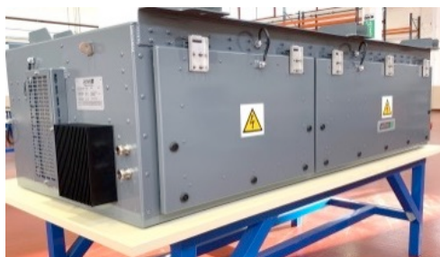
Auxiliary power converter
